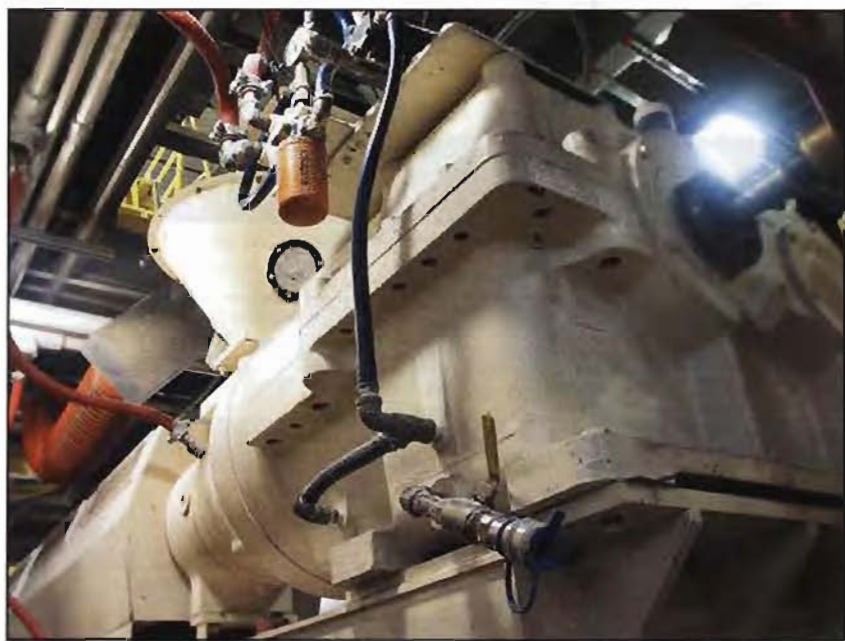
Figure 1. Quick-connect on Gear Box
